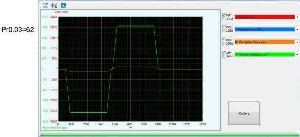
As keep decreasing the value pf Pr0.03, the position loop gain Kp become bigger and bigger, the integration time constant Vi become smaller and smaller, the position error become close to zero. Pr0.03=61
