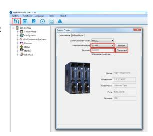
1.2.3 Click "Run Testing", and tune Pr0.04 inertia ratio and Pr0.03 stiffness, click "download" to save modified parameters, finally click "Servo Enable" to start JOG trail.
