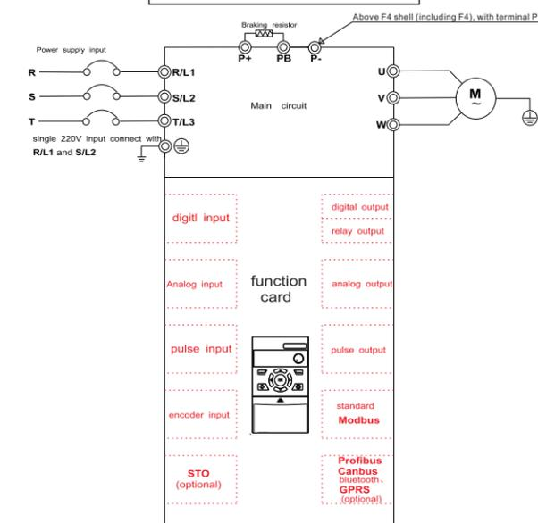
Notice: different function card corresponding to different terminals. Except standard function card, can customize any type of card. Reset parameters when using different function cards. An AC drive only can use one function card.
